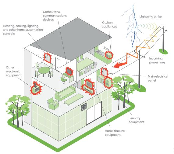
Though the odds of lightning striking your home directly are slim, the truth is that one bolt need simply touch down near the electrical supply system, even quite far away, to be just as destructive to sensitive devices connected to any power outlet.
