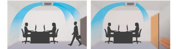
Energy saving operation commences when there are no occupants by linking up with the human sensor option. The unit will adjust its operation depending on the presence of occupants within a given room. The human sensor detects movement and activates or deactivates energy saving mode accordingly.
