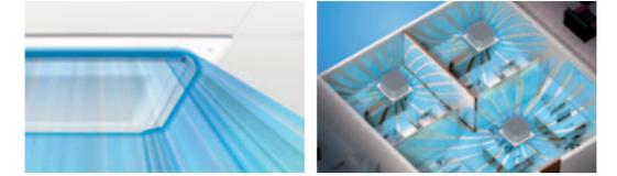
Each louver can be set individually by the controller\* to protect people from being exposed to direct airflow.
