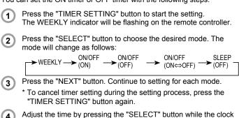
4 Adjust the time by pressing the "SELECT" button while the clock indicator is blinking. Each time you press the button, the time will change by +5/-5 minutes. Pressing down will change the time by +10/-10 minutes.
