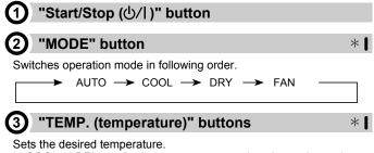
In COOL or DRY mode, the temperature needs to be set lower than the current room temperature.
