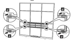
Remove dust by using a vacuum cleaner or by washing the filter. When you wash the filter, use neutral household detergent and warm water.
