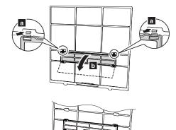
Attach new or maintained air cleaning filter d to the filter holder. New air cleaning filter can be attached to either of the right holder or the left holder.
