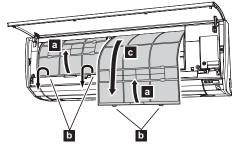
Filter holder and air cleaning filter are attached on the rear side of the air filter. Remove them from the air filter by unlatching each corner of the filter holder d.
