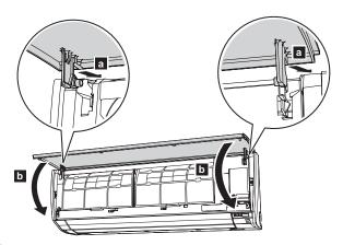
Press 4 places on the intake grille to close it completely.
