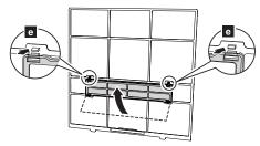
Reinstall the air filter. (Refer to step 6 in "Cleaning the air filter".)
