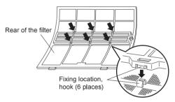
Install the two air filters and close the intake grille.
