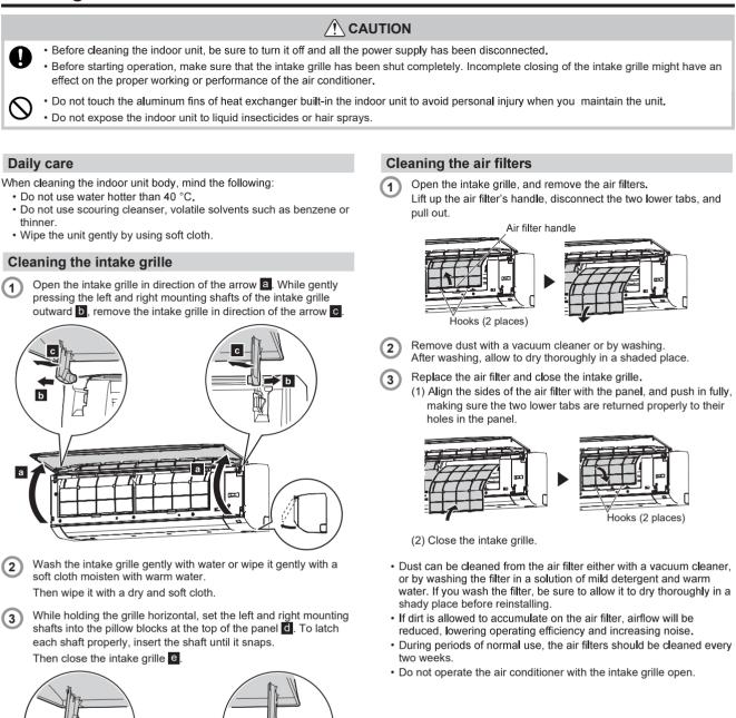
Press 4 places on the intake grille to close it completely.
