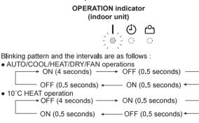
The indicator will keep blinking until the unit finishes the function.
