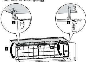
Press 4 places on the intake grille to close it completely.
