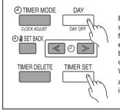
Press the DAY (DAY OFF) button and TIMER SET button simultaneously for 2 seconds or more to activate the child lock function and lock all of the buttons on the remote controller except the START/STOP button, SET TEMP. buttons, MODE button, and FAN button. Press the buttons again for 2 seconds or more to deactivate the child lock function.
