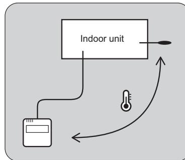
Press the ECONOMY button for more than 2 seconds to select whether the room temperature is detected at the indoor unit or the remote controller.
