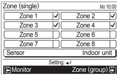
Select desired sensor with pressing the [Cursor button (Up/Down)].
