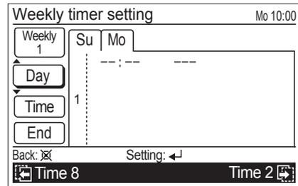
5. Set the desired conditions on the timer, such as time setting of On/Off timer, On/Off, operating mode (only for the On timer), and temperature (only for the On timer), up to 8 patterns per selected day.
