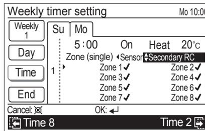
Select applicable zone name with the [Cursor button (Left/Right)], and press the [Cursor button (Up/Down)] to mark a check.
