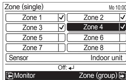
To cancel the air conditioning, set the cursor to the zone marked with a check, and press the [Enter button] to remove the check mark. Unchecked zone is not air-conditioned.
