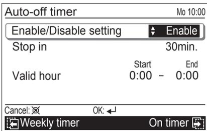
4 For [Stop in], adjust the timer with the [Cursor button (Up/Down)]. To complete the setting, press the [Enter button].
