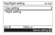
2 Select [Day setting] for the registration of group "Day", and select [Night setting] for the registration of group "Night", with the [Cursor button (Up/Down)]. When you press the [Enter button], registerable zones and roomtemperature sensor are displayed.
