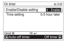
For [Time setting], adjust the time with the [Cursor button (Up/Down)], and press the [Enter button] to complete the setting.
