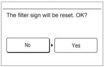
2 Select [Yes] or [No] with the [Cursor button (Left/Right)], and press the [Enter button]. When [Yes] is selected, the filter sign icon on the display is turned off.
