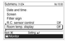
2 Select [On] or [Off] with the [Cursor button (Up/Down)], and press the [Enter button].
