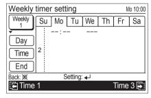
3. Press the [Enter button]. Then select [Weekly 1] or [Weekly 2] with the [Cursor button (Up/Down)], and press the [Enter button].
