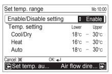
**4** For [Temp. setting], select mode with the [Cursor button (Up/Down)] and press the [Enter button].
