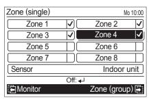
To cancel the air conditioning, set the cursor to the zone marked with a check, and press the [Enter button] to remove the check mark. Unchecked zone is not air-conditioned.
