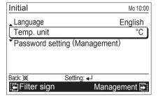
2 Select [°C] or [°F] with the [Cursor button (Up/Down)] and press the [Enter button].
