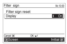
When you set this setting to [On], and air filter cleaning on the indoor unit is required, the icon is displayed on the "Monitor" screen.
