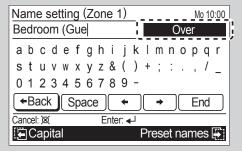
Set the cursor to [End] with the [Cursor button], and press the [Enter button] to finalize the name registration.
