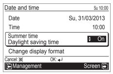
To complete the setting, press the [Enter button]. Screen returns to the "Date and Time" screen.
