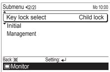
Select [Child lock] or [Part lock] with the [Cursor button (Up/Down)], and press the [Enter button].
