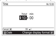
To complete the setting, press the [Enter button]. The screen returns to the "Date and Time" screen.
