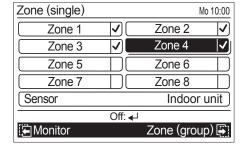
To cancel the air conditioning, set the cursor to the zone marked with a check, and press the [Enter button] to remove the check mark. Unchecked zone is not airconditioned.
