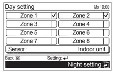
Select the room-temperature sensor with the [Cursor button (Up/Down)].
