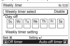
Select any of [Weekly 1], [Weekly 2], or [Disable] with the [Cursor button (Up/Down)], and press the [Enter button].
