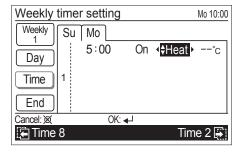
(6) When you selected [On] (On timer), adjust the value to the desired temperature with the [Cursor button (Up/ Down)].
