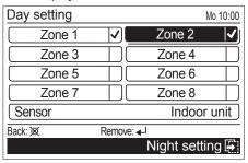
To remove the check mark, adjust the cursor to the zone name to be unchecked, and press the [Enter button] again.
