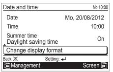
"Change display format" screen is displayed. Select the setting items (Date format or Time format) with the [Cursor button (Left/Right)] and set with the [Cursor button (Up/Down)].
