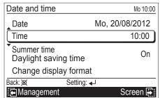
"Time" screen is displayed. Select the setting items (hour, min., or AM/PM) with the [Cursor button (Left/Right)] and set with the [Cursor button (Up/Down)]. When setting the minutes, setting can be completed quickly if the button is pressed continuously.
