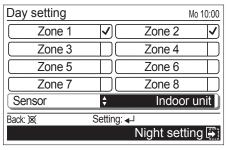
Each time you press the [Cursor button (Up/Down)], displayed sensor switches as follows. Non-connected sensor will be skipped.
