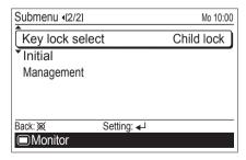
2 Select [Child lock] or [Part lock] with the [Cursor button (Up/Down)], and press the [Enter button].
