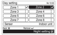
To remove the check mark, adjust the cursor to the zone name to be unchecked, and press the [Enter button] again.
