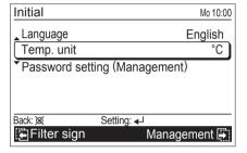
2 Select [°C] or [°F] with the [Cursor button (Up/Down)] and press the [Enter button].
