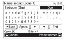
**4** Set the cursor to [End] with the [Cursor button], and press the [Enter button] to finalize the name registration. Screen returns to the "Name setting" screen, and registered name is displayed.
