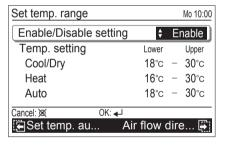
**4** For [Temp. setting], select mode with the [Cursor button (Up/Down)] and press the [Enter button].
