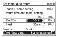
To complete the setting, press the [Enter button]. To return to the "Function" screen, press the [Cancel button].
