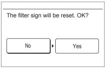
2 Select [Yes] or [No] with the [Cursor button (Left/Right)], and press the [Enter button]. When [Yes] is selected, the filter sign icon on the display is turned off.
