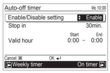
4 For [Stop in], adjust the timer with the [Cursor button (Up/ Down)]. To complete the setting, press the [Enter button].
