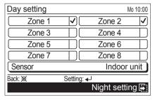
2. Select the room-temperature sensor with the [Cursor button (Up/Down)].
